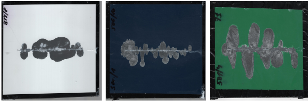
Test specimen removed from salt fog chamber.
