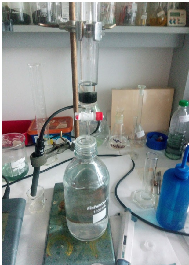
Figure 4: Column arrangement of experiments to determine the total capacity of the strongly acidic cathexis Lewatit Mono Plus S108
