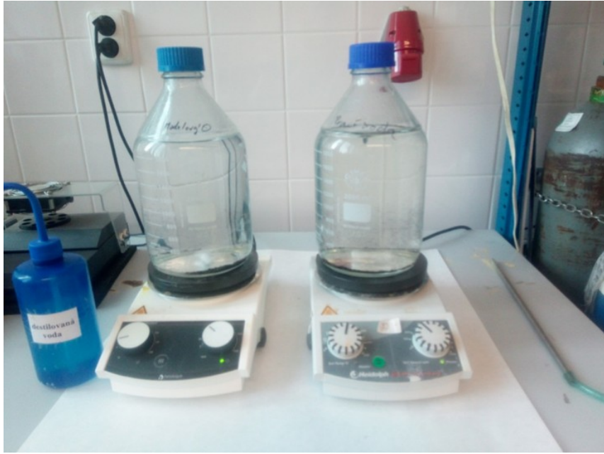
Figure 3: Batch arrangement of experiments to determine the total capacity of the strong acid cathexis Lewatit Mono Plus S108
