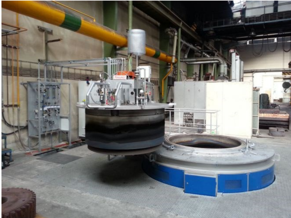
Obr. 1.7 – Hlubinná pec (Realistic, 2015)
