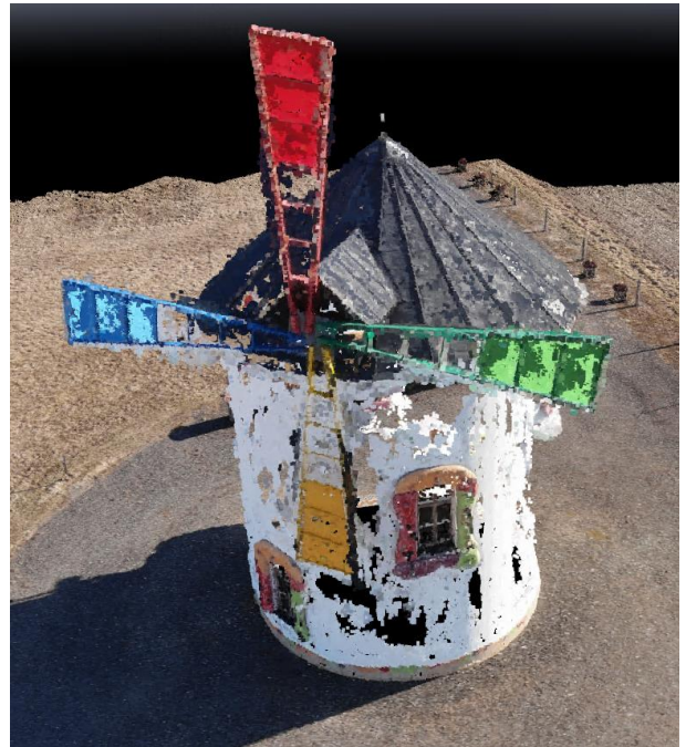
Figure 7. Detail of 3D model from Pix4Dmapper – point cloud
