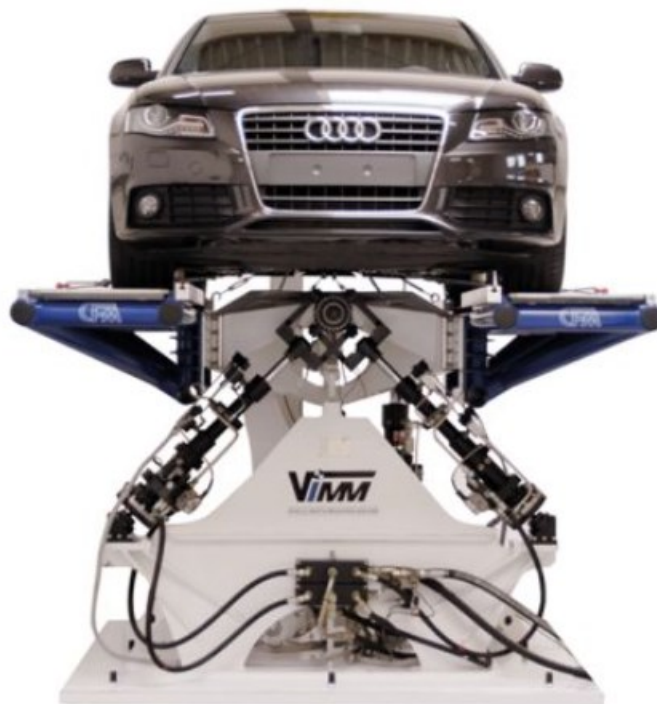
Obrázek 18: Vehicle inertia measuring machine, CFM Schiller [19]
