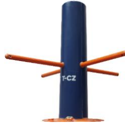
Fig. 2. Train antenna employed for the optical detection when the object passes by the reference point.
