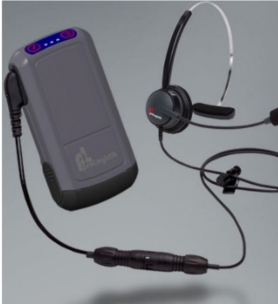
Obrázek 22 Kapesní stanice a sluchátka pro systém Pick by Voice (Easyfairs Group, ©2019)
