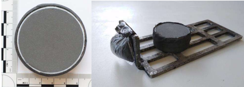
Fig. 1 Detailed sample of propellant (left) sample on iron grid holder with attached bag of black powder (right).
