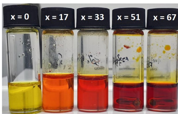
Figure 1 – Chalcogenide glass solutions of As_{33}S_{67-x}Se_x glass system prepared by mixing binary solutions of As_{33}S_{67} and As_{33}Se_{67} chalcogenide glass.
