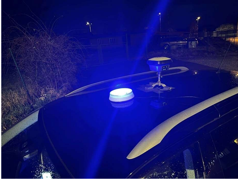
Figure 33 The mounted GNSS on the car, with the marked light to easier identify it.
