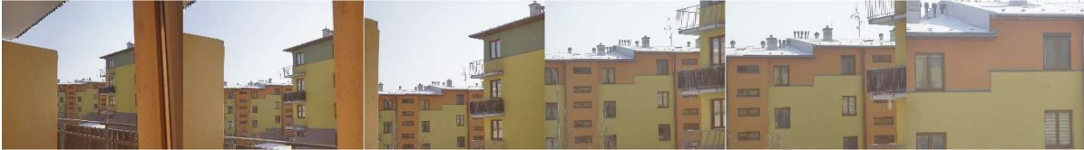
Figure 9 An illustration of different focal lengths from the right 24 mm, 35 mm, 55mm, 80 mm, 105 mm, 200m the photo was captured from the same spot and the zooming is due to optical effect
