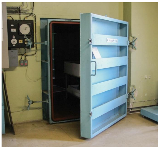
obr. 37 Ethylénoxidová komora Fumigation System VSF 250 firmy Vacudyne Altair v SNA
