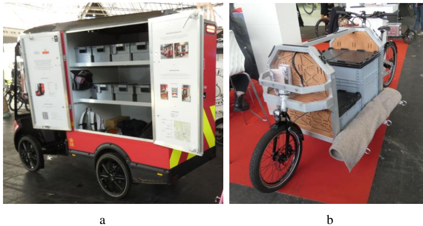
Fig. 1 Cargo bikes with the possibility of dividing a cargo space: a – four-wheeler; b – two-wheeler.
