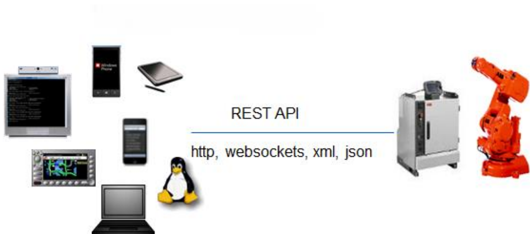
Obrázek 3.8 – Robot web Services (Application manual– Robot Web Services, 2020)
