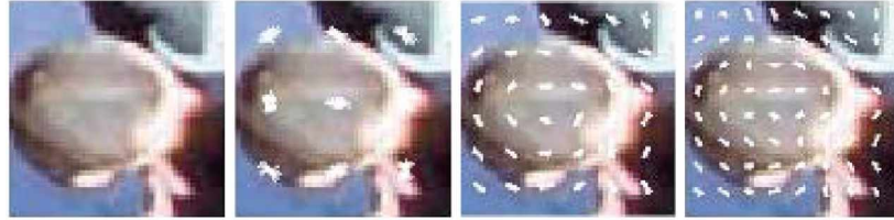
Figure 9 – Images with highlighted HOG features for different cell sizes. Taken from (Stursa, 2020a).
