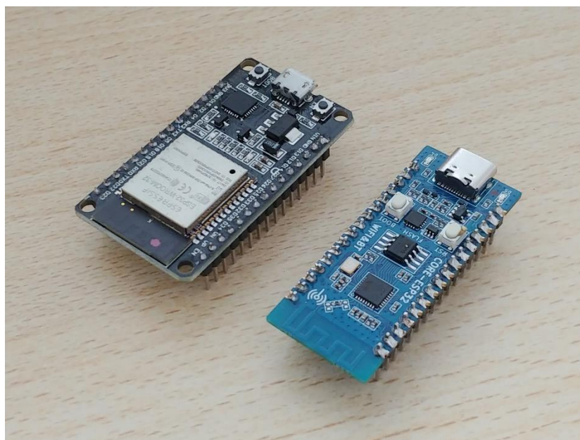
obr. 6 - vlevo ESP32 DevKit, vpravo ESP32 C3 AIRM2M CORE
