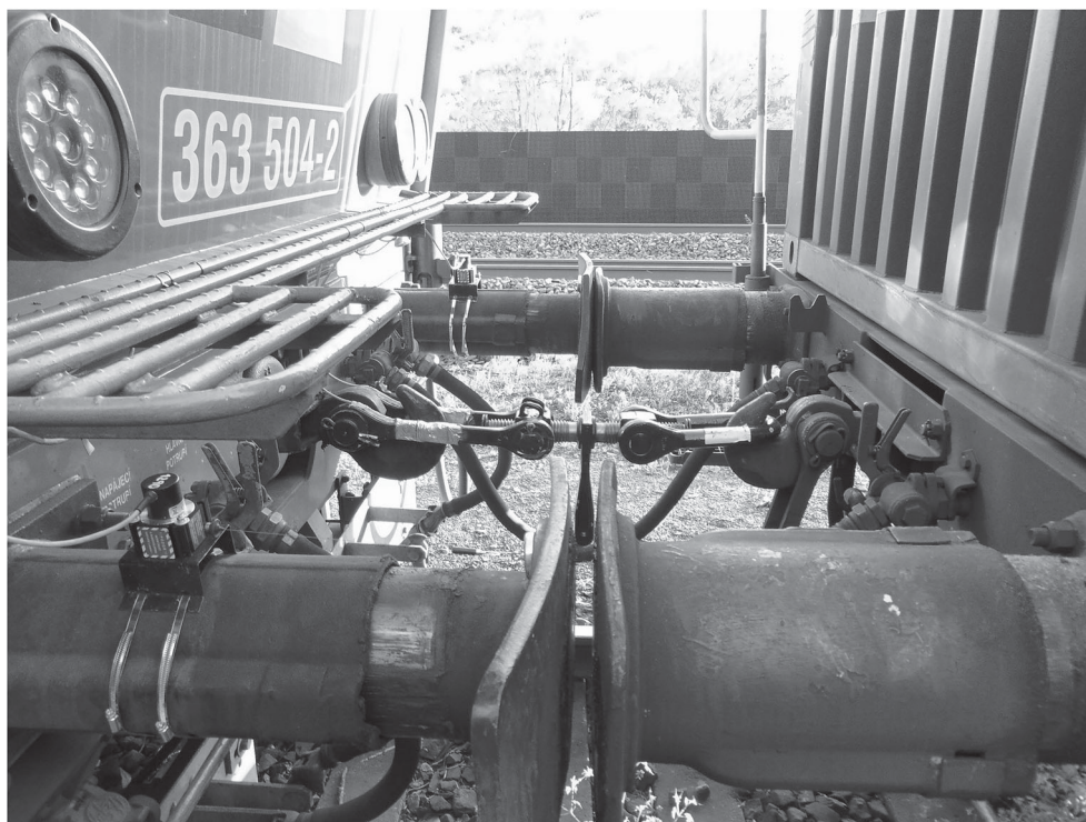
Figure 2. Connection of the locomotive and the first wagon by the instrumented screw coupling; the length sensors measuring compression of the locomotive buffers are also visible.
