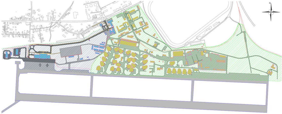
Figure 12 - layout of the airport (military compound buildings shown in beige, military area in green hatching, civil airport buildings in light blue and civil airport area in blue hatching)
