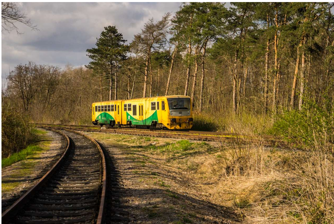
Image 12 - view north from the compound entrance showing ČD class 814 "Regionova" on the 237 line, a type of train unit, that could operate on the extension of the branch line, since the unit has crew compartments on both front and rear of the unit.
