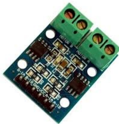
Obr. 2.14 – Driver L9110S (L9110 2-CHANNEL MOTOR DRIVER, 2021)
