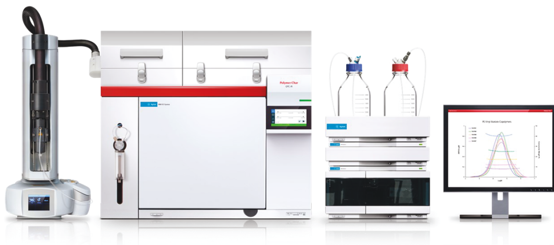
Figure 24 Photo of high-temperature size exclusion chromatography coupled with a filter-based multiple band IR detector (IR5).
