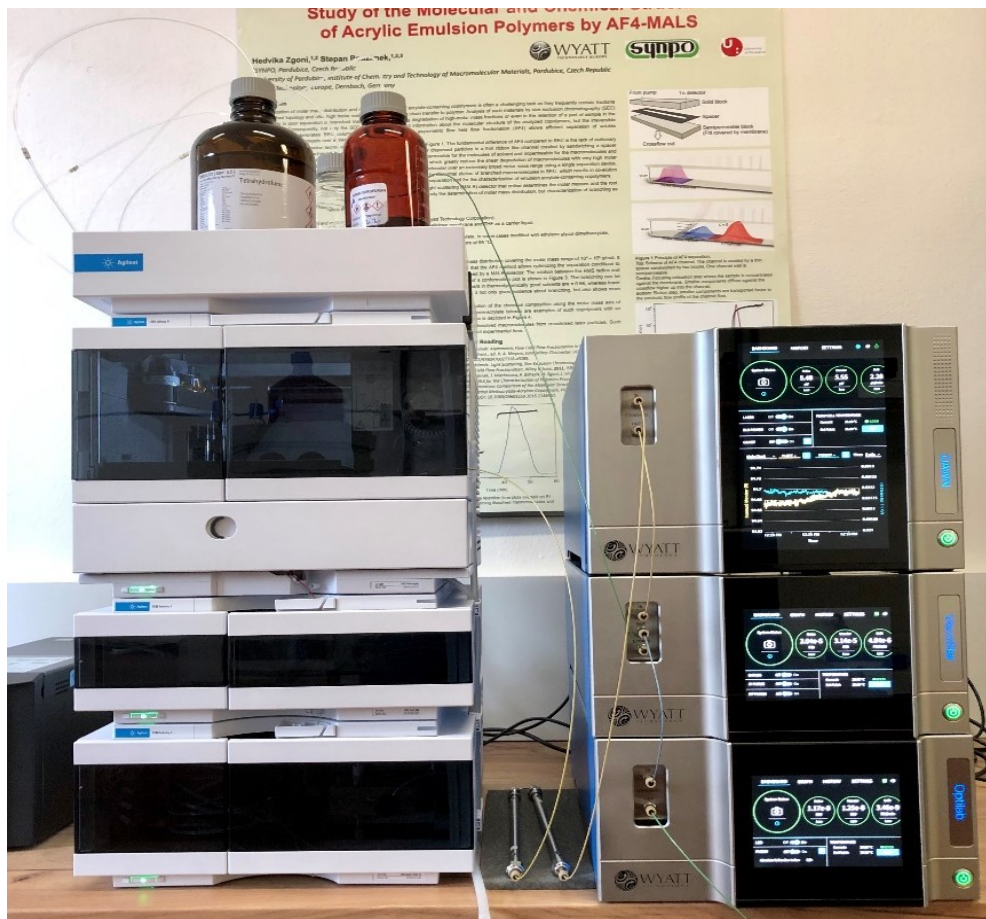
Figure 4 Photo of size exclusion chromatography coupled with multi-angle light scattering and an online viscometer.
