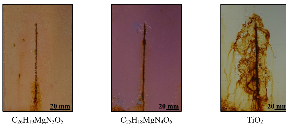
Fig. 6 Epoxy ester coatings containing TiO 2 and tested pigments at PVC = 3 % after 1440hour exposure in an atmosphere containing salt fog
