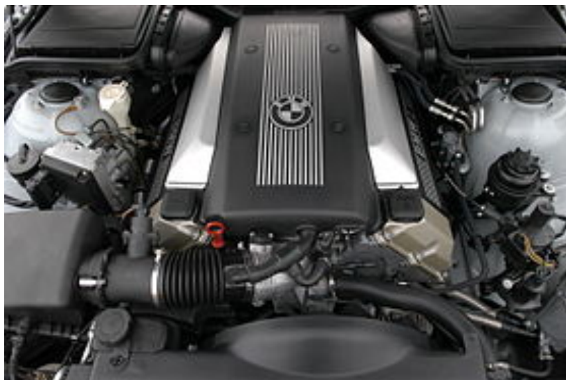
obr. 5: Motor BMW M62B44 [7]
