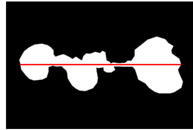
Fig. 4 White area is the area of delamination, the scribe is marked by red
