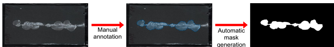
Fig. 5 The Delamination Labeler - a custom-made application for data annotation
