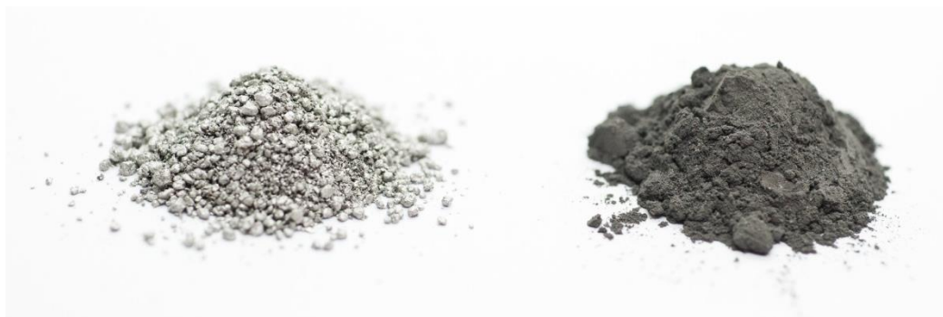
Figure 11. Effect of methanol addition on mechanically activated aluminum-nickel metal mixture – 0 wt.% left, 5 wt.% right (photo by Bc. Andrea Hegedüs).
