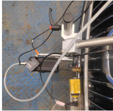
Figure 4– An optical gate sensor: Balluff BOS 36K-PA-1QH-S 4-C
