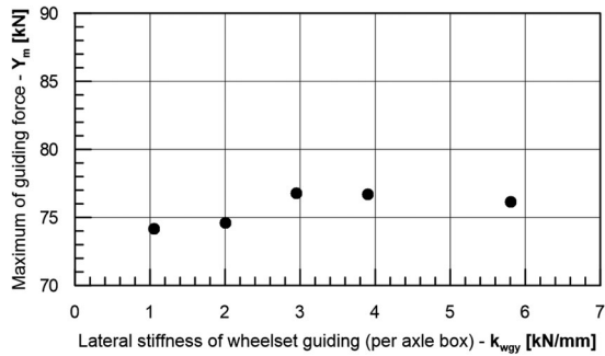
Figure 6. Maximum value of guiding force of the four-axle locomotive model in the S-curve in dependency on the lateral stiffness of wheelset guiding (for the longitudinal stiffness value of ca. 90 kN/mm).
