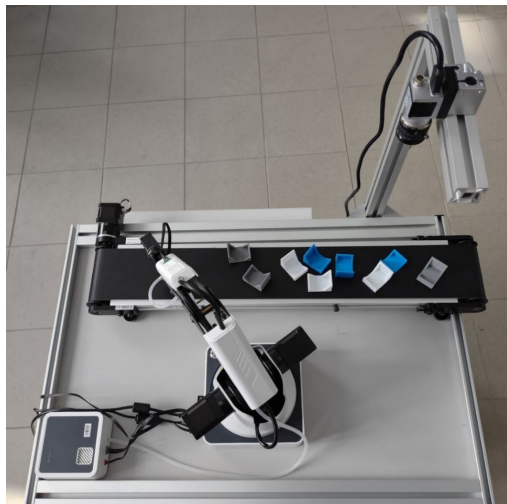
FIGURE 17. A demonstrative robotic stand for data acquisition. Objects of interest are scattered on a conveyor belt. An industrial camera situated above the scene is used for RGB image acquisition. A line LED light is situated in the aluminium profile near the camera.
