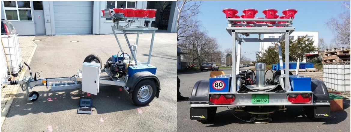
Figure 10 falling weight deflectometer device, different views
