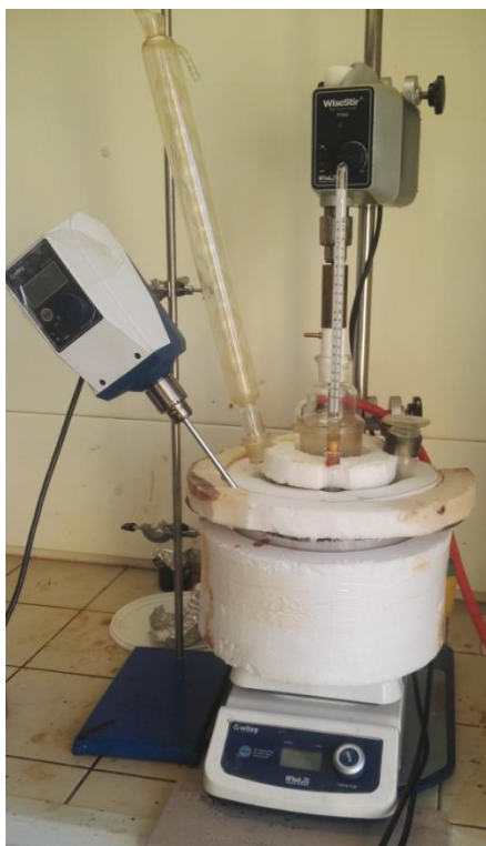
Fig. 5: Apparatus for partial flexible PUR foam depolymerisation: oil bath, reflux condenser, nitrogen gas inlet, and high-torque mixer
