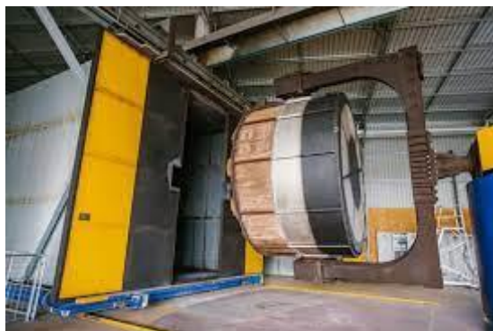
Obr. 27 Forma a pec pro rotomoulding [46]
