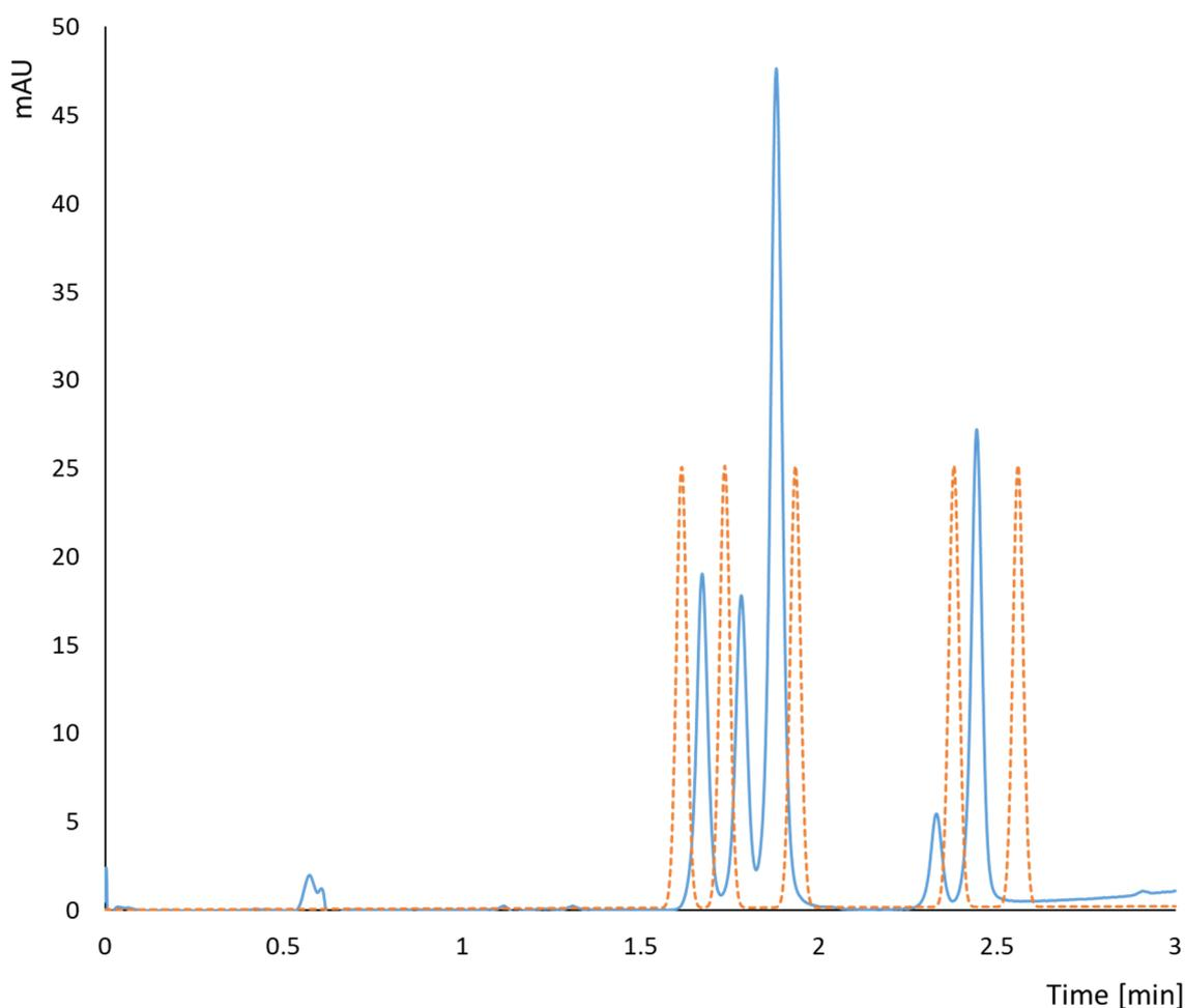
**Fig. 3** Fast gradient separation benzodiazepines – comparison of experimental (full line) and predicted (dotted) chromatograms
