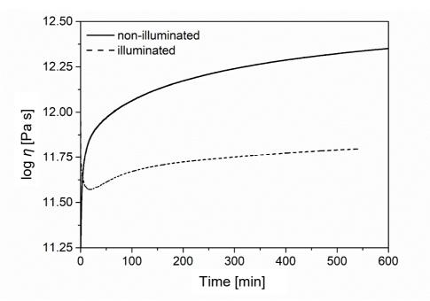
Fig. 4 Comparison of viscosity measurements of non-illuminated and illuminated  $(\lambda = 650 \text{ nm}, F_L = 2.1 \text{ W/cm}^2)$  samples of As<sub>2</sub>S<sub>3</sub> glass measured at 178 °C
