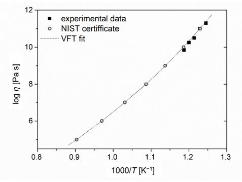
Fig. 2 Viscosity data for viscosity standard SRM 717a: (■) our data measured by penetration method employing modified thermomechanical analyzer and (○) the tabulated data [17] plotted versus reciprocal temperature The tabulated data are fitted by VFT equation (2)
