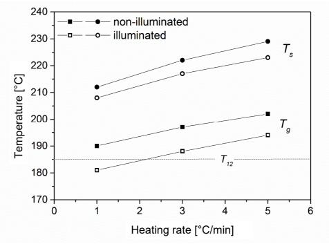
**Fig. 6** The change of characteristic temperatures (glass transition temperature  $T_g$  and softening temperature  $T_s$ ) obtained from dilatometric curve for non-illuminated and illuminated As<sub>2</sub>S<sub>3</sub> ( $\lambda = 650$  nm,  $F_L = 2.1$  W/cm<sup>2</sup>) as a function of heating rate Dashed line corresponds to value of the viscosity glass transition temperature  $T_{12}$  determined from viscosity measurements.
