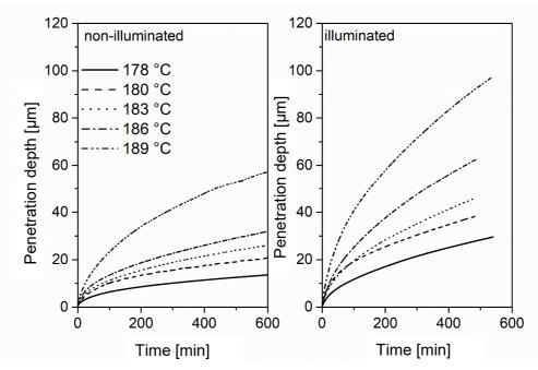
Fig. 5 Time dependence of *h* of non-illuminated and illuminated ( $\lambda = 650 \text{ nm}, F_L = 2.1 \text{ W/cm}^2$ ) samples of As<sub>2</sub>S<sub>3</sub> glass measured at different temperatures
