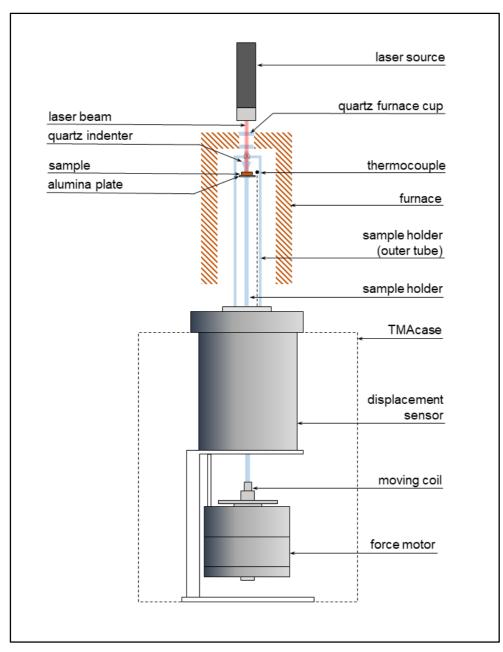
**Fig. 1** Schematic outline of the thermomechanical analyzer TMA CX 03RA-T adapted for the study of photoinduced changes on viscous flow
