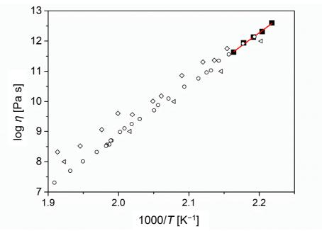
Fig. 3 The temperature dependence of logarithms of viscosity (logη) of A<sub>2</sub>S<sub>3</sub>: our data (■), Hofírek [11] data (○), Málek [9] data (◊), and Nemilov [10] data (⊲) The solid line corresponds to linear fit of our data.
