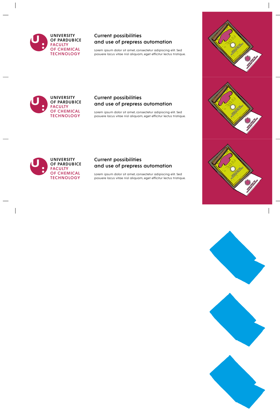
Fig. 156: Example of resulting a) printing data, b) data for varnishing (see Fig. 34) processed by the workflow presented in Fig. 146 in Esko Automation Engine 18.1.0 (scale 1 : 2)
