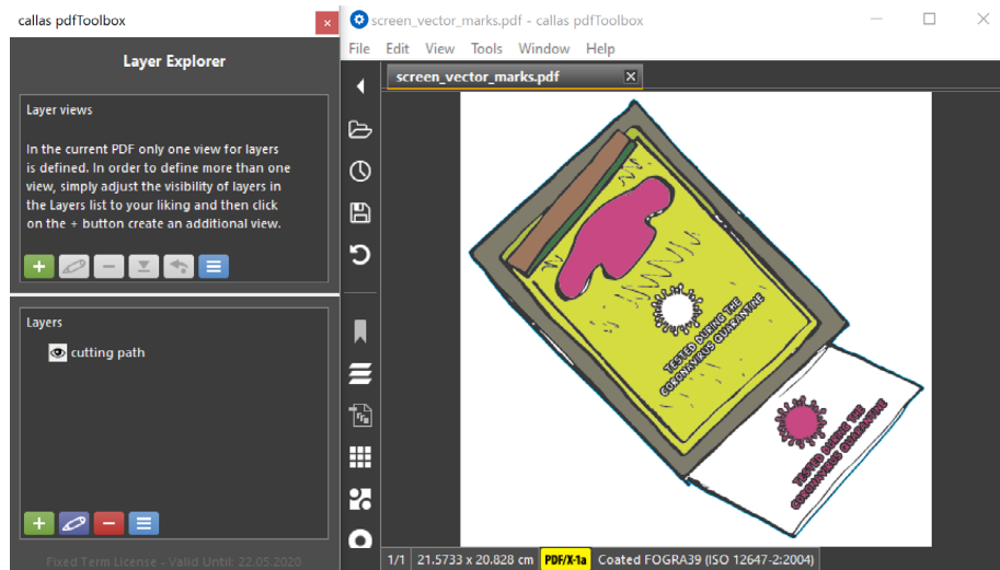
Fig. 82: Modified printing data with the created layer named “cutting path” defining a path for cutting in Callas pdfToolbox Desktop 11
