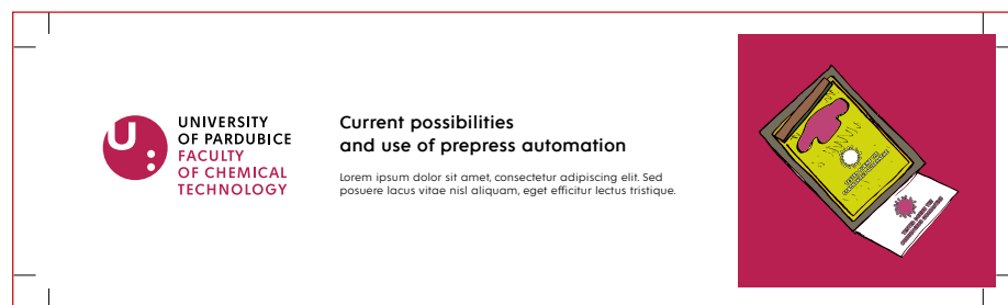
Fig. 43: A preview of the printing data fixed according to the assumed requirements (content with the bleed and trim marks and the corresponding size of the CropBox) using the action in Adobe Acrobat X Pro (scale 1 : 2), the CropBox marked with a red line
