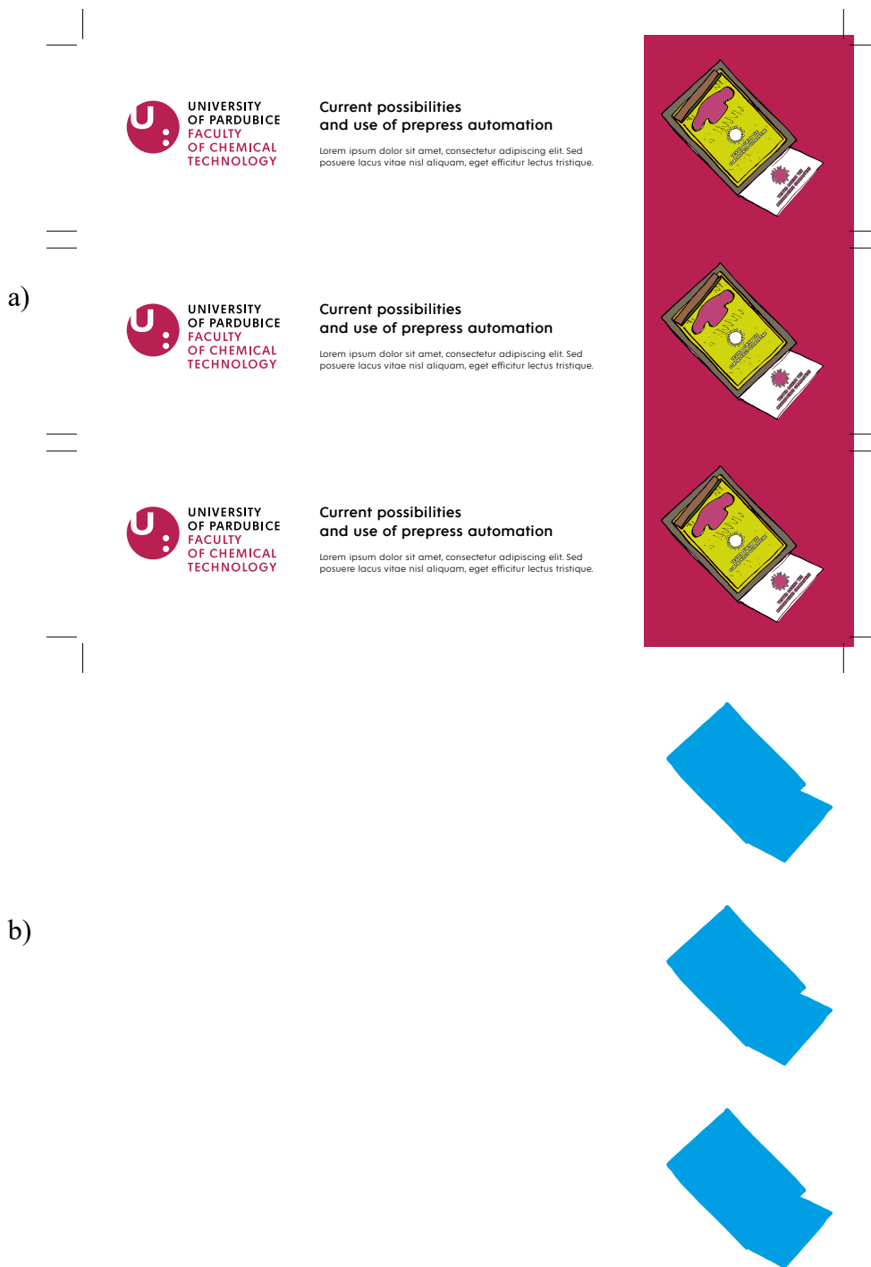
Fig. 78: Example of the resulting a) printing data, b) data for varnishing for the first and second printing data (see Fig. 34 and Fig. 35) processed by the workflow presented in Fig. 77 and Fig. 76 in Callas pdfToolbox Desktop 11 (scale 1 : 2)
