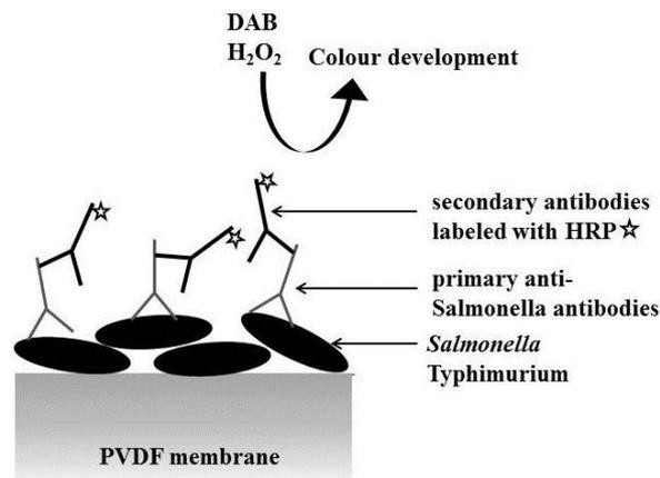
Fig. 1 Scheme of whole-cell dot blot method
