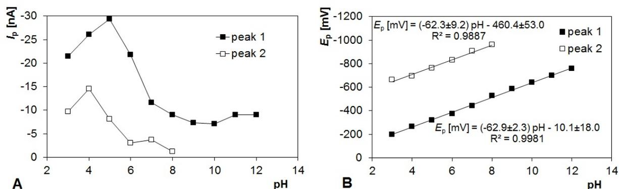
Fig. 3 Dependence of current response (A) and peak position (B) of  $1 \times 10^{-5}$  mol  $\text{l}^{-1}$  MTX on pH value of supporting electrolyte recorded on p-AgSAE. Method: CV; parameters:  $E_{in} = 0$  mV,  $E_{fin} = -1300$  mV,  $\nu = 100$   $\text{mV s}^{-1}$ . Supporting electrolyte: BR buffer of pH from 3 to 12
