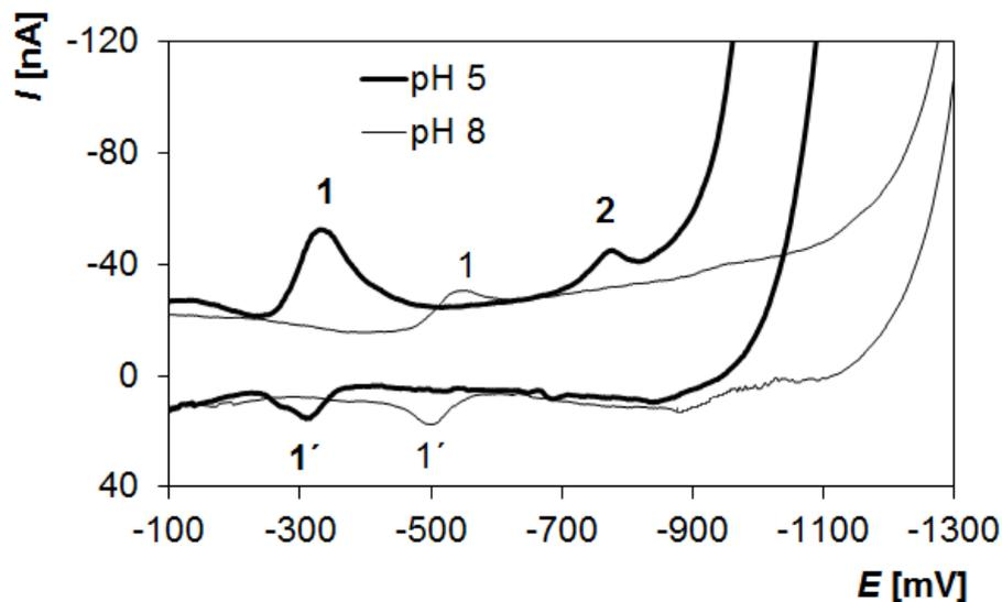
Fig. 2 Cyclic voltammogram of  $1 \times 10^{-5}$  mol  $\text{l}^{-1}$  MTX in BR buffer of pH 5 and 8 recorded on p-AgSAE. Method: CV; parameters:  $E_{in} = 0$  mV,  $E_{fin} = -1300$  mV,  $\nu = 100$   $\text{mV s}^{-1}$ . Legend: 1, 2 – reduction signals of MTX, 1' – oxidation signal of MTX
