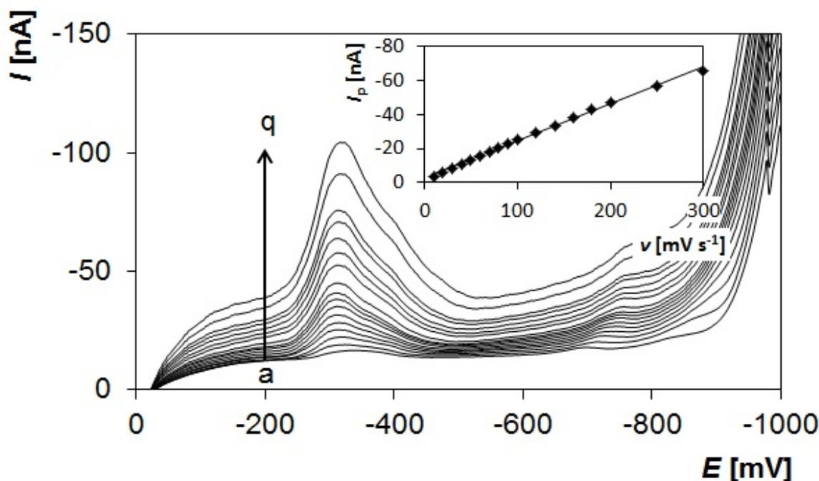
Fig. 4 Voltammetric curves of  $5 \times 10^{-6} \text{ mol l}^{-1}$  MTX at different scan rates obtained on p-AgSAE. Method: DCV; parameters:  $E_{in} = 0 \text{ mV}$ ,  $E_{fin} = -1000 \text{ mV}$ ,  $\nu = 10\text{--}300 \text{ mV s}^{-1}$ ; supporting electrolyte:  $0.05 \text{ mol l}^{-1}$  acetate buffer (pH 5). Legend: a – 10, b – 20, c – 30, d – 40, e – 50, f – 60, g – 70, h – 80, i – 90, j – 100, k – 120, l – 140, m – 160, n – 180, o – 200, p – 250 and q –  $300 \text{ mV s}^{-1}$
