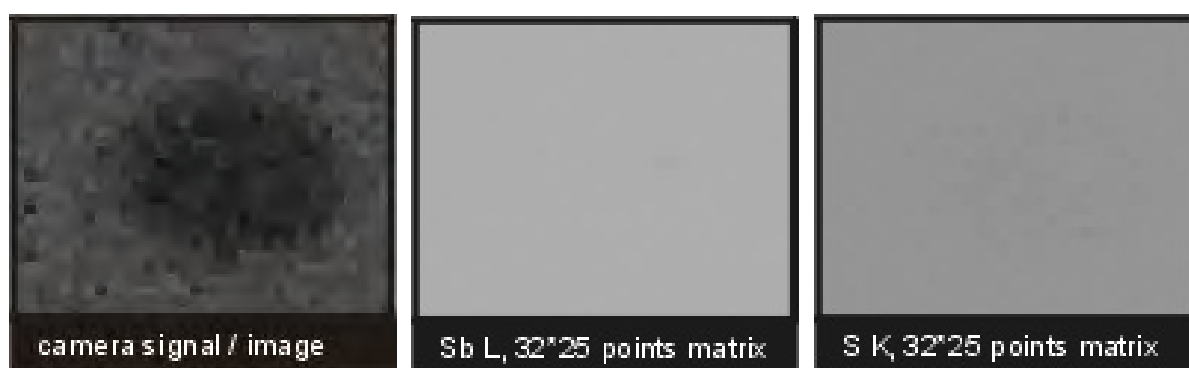
Fig. 5 XRF compositional maps together with image of analyzed laser exposed dot ( t_{\text{EXP}} = 20 s) of b2-0 sample
