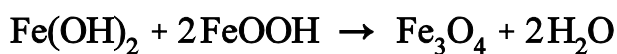
Fig. 1 The principle of preparation of magnetic nanoparticles of \text{Fe}_3\text{O}_4 by oxidation method
