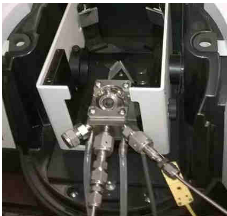
Fig. 1 Praying Mantis diffuse reflectance accessory. Experimental set-up
