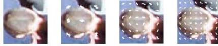
Fig. 3. HOG features for 9 bins and cell size [16, 16] px, [8, 8] px and [6, 6] px. Original size of the object image is [51, 51] px. The length of white abscissae is related to the gradients in the image.
