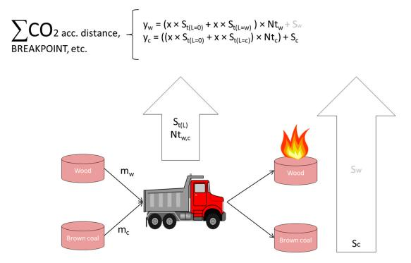
**Figure 1.** Illustration of process of the total CO<sub>2</sub> emission evaluation for transport and combustion together. Source: own processing.
