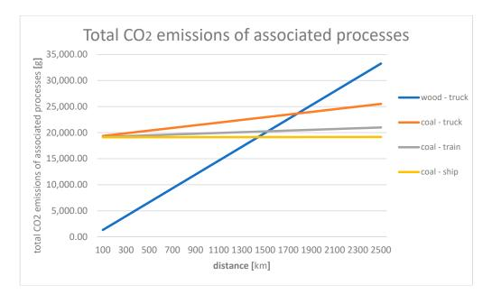
**Figure 3.** Total CO<sub>2</sub> emissions of associated processes of selected fuels and related break points. Source: own processing.
