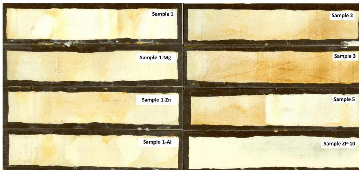
Figure 11 Appearance of steel sheets of all tested samples after an accelerated corrosion test
