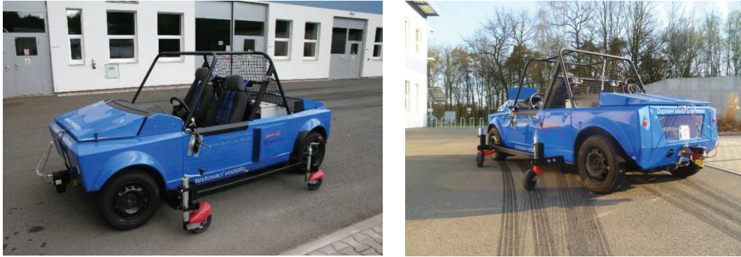
Fig. 1 The experimental car with the alternative SkidCar system
