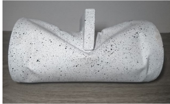
Fig. 4 Deformed experimental model at the end of the loading.
