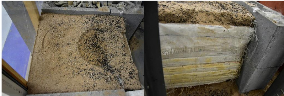
Figure 6.5 Pictures of wall with sand backfill and 10% tyre crumb after failure
