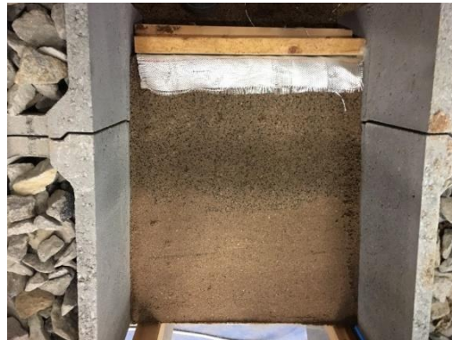
Figure 6.3 Overlapping length of geotextile
