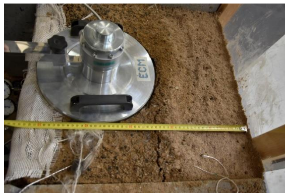
Figure 6.14 Failure Cracks of Clay + 10% Tyre Crumb Mixture
