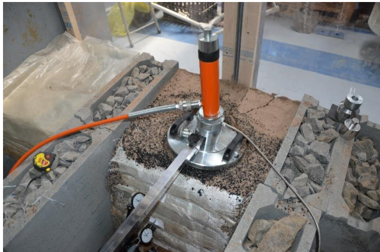
Figure 6.8 Failed wall for sand and 30% tyre crumb mixture after application of 0.24 MPa load
