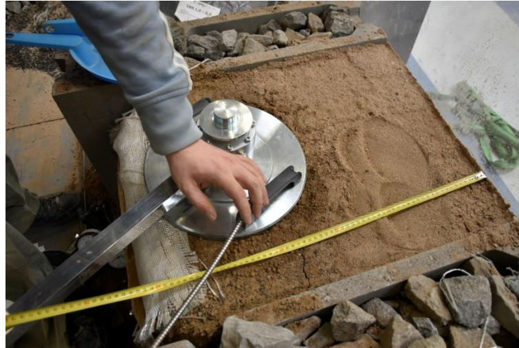
Figure 6.15 Failure cracks of Clay + 20% Tyre Crumb Mixture
