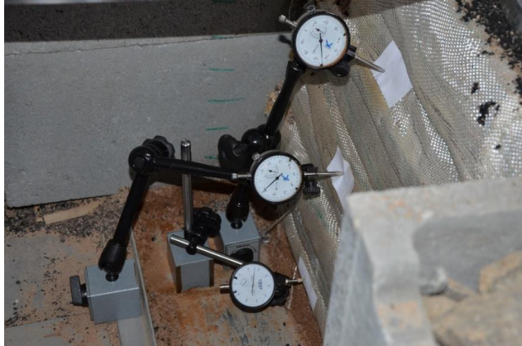
Figure 6.7 Location of measurement points of horizontal displacement
