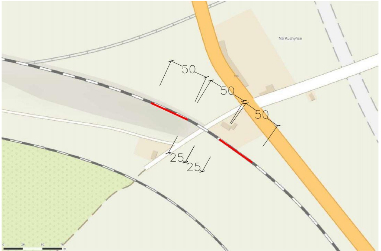
Figure 32 - Marking of survey sections in the area of railway crossing number 8
