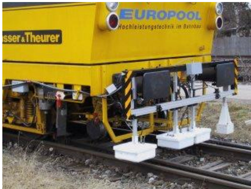
Figure 13 - Antenna position in front of the locomotive [35]
