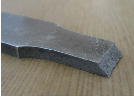
Fig. 9.3. Specimen of an Al alloy after tensile test. Width 11 mm, thickness 3 mm.
