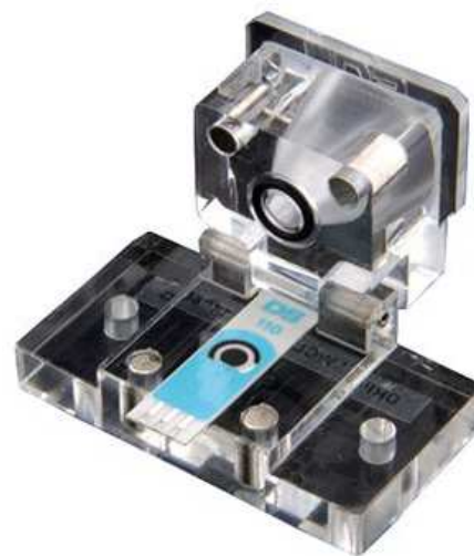
Fig. 1. Methacrylate (transparent) wall-jet flow cell for FIA.
