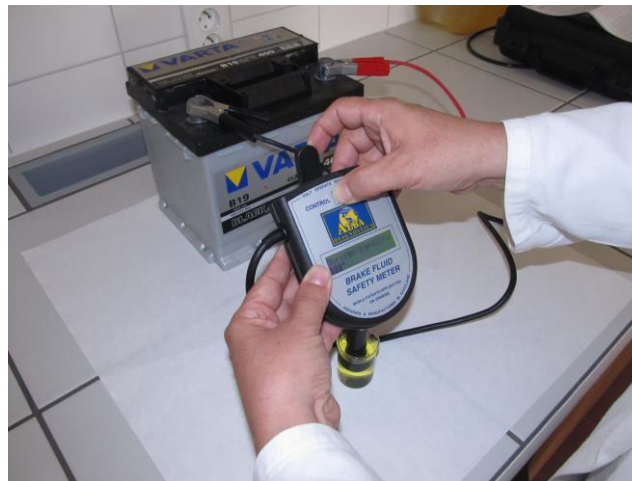
Fig. 1 Measure the boiling point of the brake fluid with the Alba diagnostics
