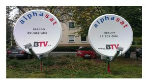
Fig.1. The 19 GHz and 39 GHz Alphasat satellite signal receivers of the Institute of Atmospheric Physics in Prague, Czech Republic
