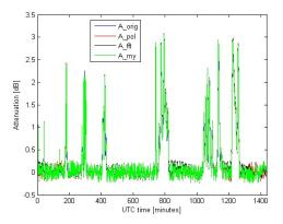
**Fig.11.** Atmospheric attenuation after application of all methods in charge while the inspiration default signal level course from Fig. 10 is used
