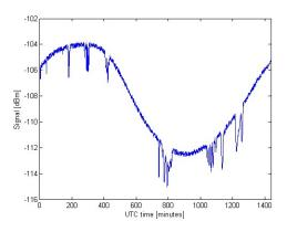
Fig.10. Other example of simulated signal level time course
