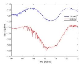
**Fig.2.** Example of 24h recorded signal level fluctuation due to satellite space motion which is the source for signal template (Prague, 6.1.2017)
