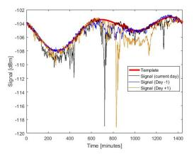
**Fig.7.** Constructed final template (red colour) after both polynomial and FFT/IFFT procedures applications (i.e. the MY method)
