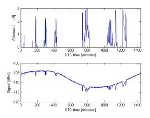
**Fig.8.** Example of simulated atmospheric attenuation time course (upper) and signal level course (below) respecting the fluctuations of received signal due to the space instability of the Alphasat satellite
