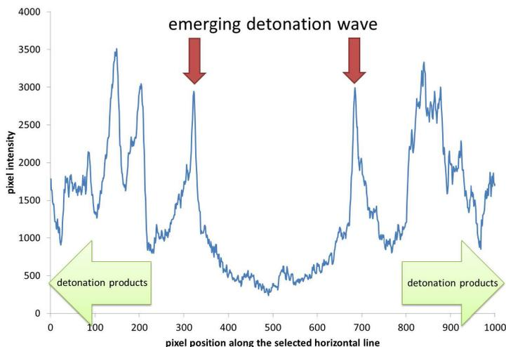
**Figure 7.** Evaluation of the position of the detonation front emerging from the face of the charge.
