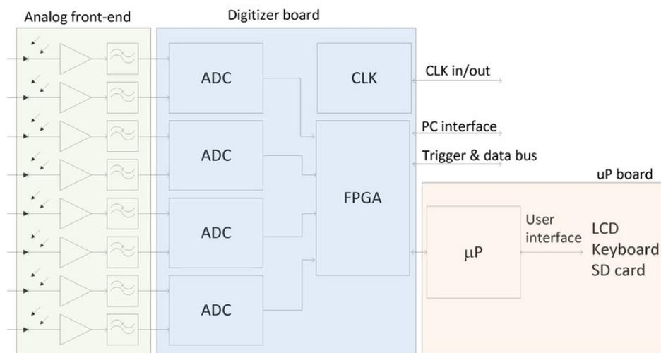
**Figure 5.** Block schematic of the 8-channel measurement system OPTIMEX.
