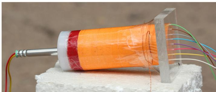
**Figure 2.** Experimental arrangement showing the positions of the blasting cup, centering ring, booster charge, the two HE pellets, trigger and the PMMA window serving as the fiber holder (variant with  $L/D=2$  and 8 optical probes evenly spaced along the charge diameter).
