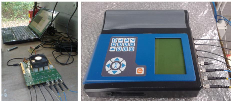
**Figure 4.** OPTIMEX 4 + 4 system during outdoor trials (left) and the final prototype of a handheld 4 + 4 version complemented with a graphical display and keyboard as a user interface (right).
