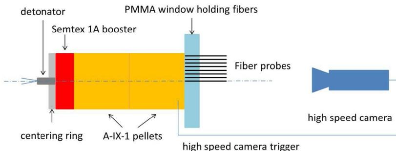
**Figure 1.** Schematic diagram of the experiment (variant with  $L/D = 2$  and 8 optical probes evenly spaced along the charge radius).
