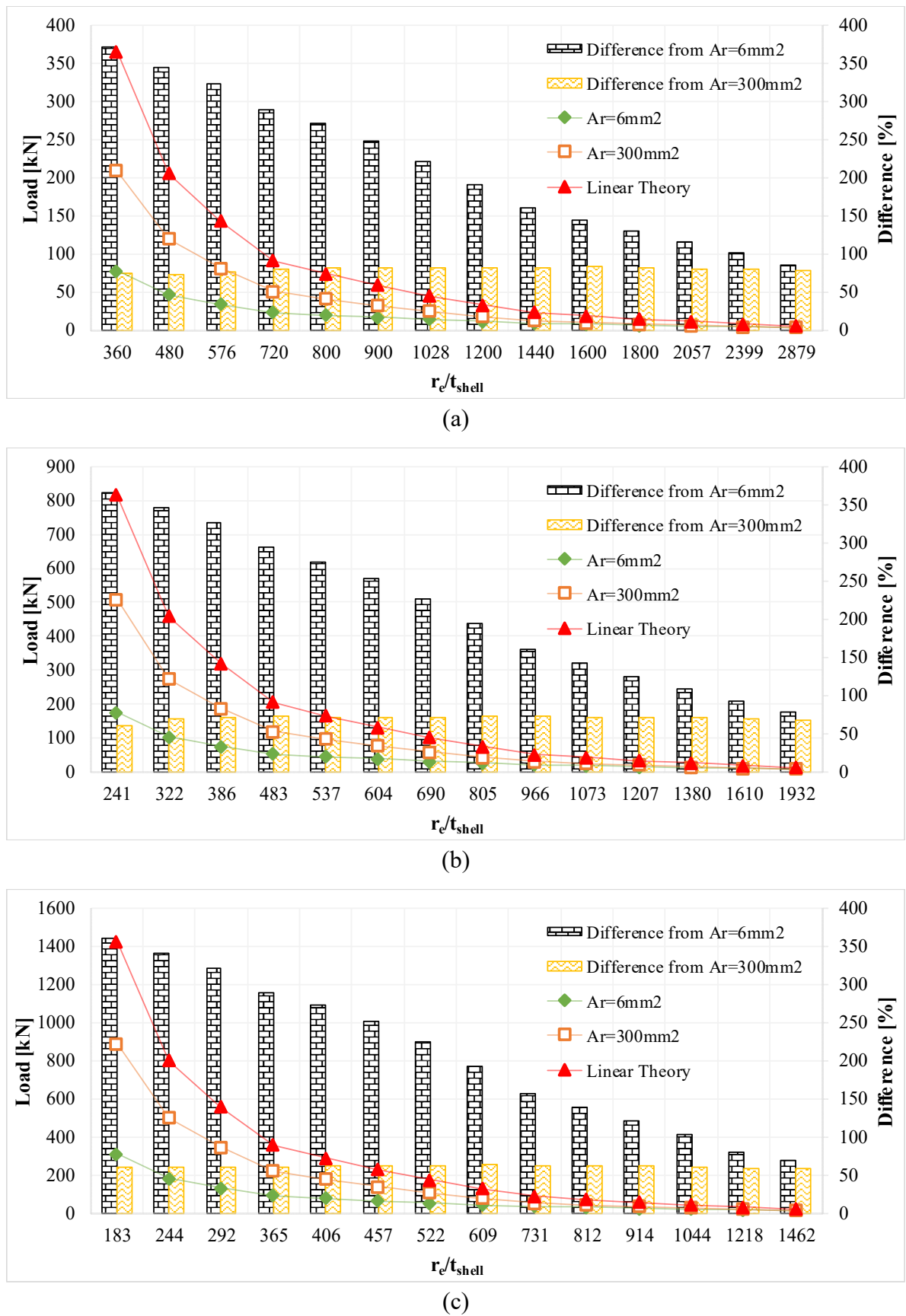
Figure 5.8. Comparison of the theoretical calculation with the limit loads of A_{ring}=6 \text{ mm}^2 and A_{ring}=300 \text{ mm}^2 cases. (a) Base angle 10^\circ , (b) Base angle 15^\circ , (c) Base angle 20^\circ .
